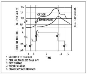
**Figure 1** – Voltage and Temperature of a Ni-Cd cell being charged with constant current. The voltage peaks when the cell is fully charged and the temperature rises. Full charge can be determined by detecting when dV/dt goes to zero or negative, or when the temperature rises. Commercial chargers use these methods to determine full charge. (From MAX712/713 data sheet)
