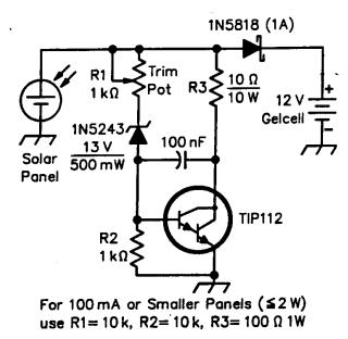
**Figure 8** – This simple charge controller will handle charging currents up to 1 A. When the battery is fully charged, all of the current from the panel will be going through R3 and the Darlington transistor TIP112, so these must be well heat sunk. Adjust R1 for the trip point, usually 14.4 V – 15 V for a 12 V SLA or a 12 V Ni-Cd battery. (From "QRP Power" p 3-24)
