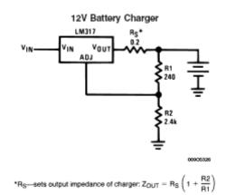
**Figure 4** – A battery charger built from an LM317 variable voltage regulator. It is advisable to place a diode between the regulator and the battery to prevent discharge of the battery if a short circuit occurs in the charger. If the charger is located far from the supply, a 0.1 uF tantalum bypass capacitors should be added to the input. The values shown are for a 13.7 V charger. For other voltages, V = 1.25(1+R2/R1). Vin should be 18 V or greater. (from LM317 data sheet)
