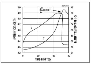
**Figure 2** – The voltage and temperature response of a Ni-MH battery being charged at constant current. The voltage maximum, indicating full charge is much shallower than it is with a Ni-Cd cell. (From MAX712/713 data sheet)
